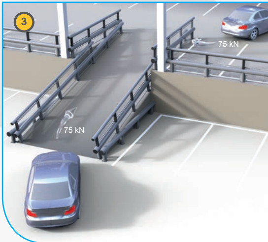
TYPICAL RAMP BARRIER CONDITION
