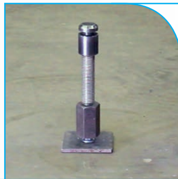
Threaded studs are used for anchorage tests
